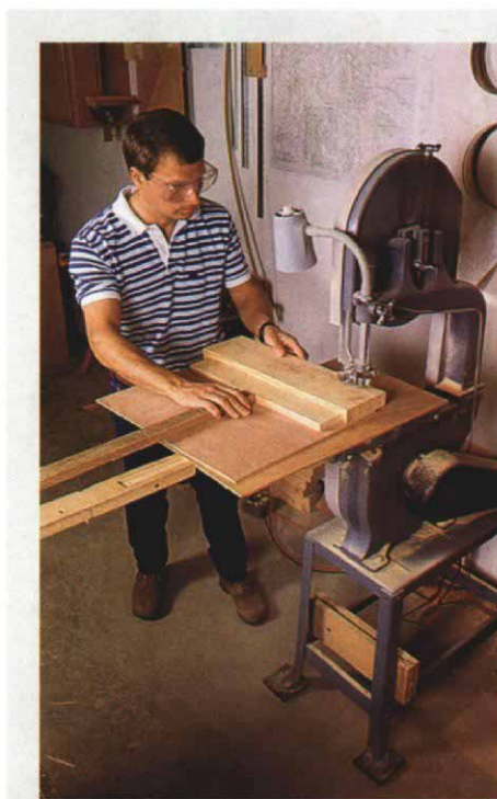
For round-top windows with small radii, Shafer cut sections of the bending forms on the simple jig shown in the drawing. For bigger windows, he attached a length of 1x3 to the plywood carriage (above) and extended it across the room to a center point on top of a workbench.
